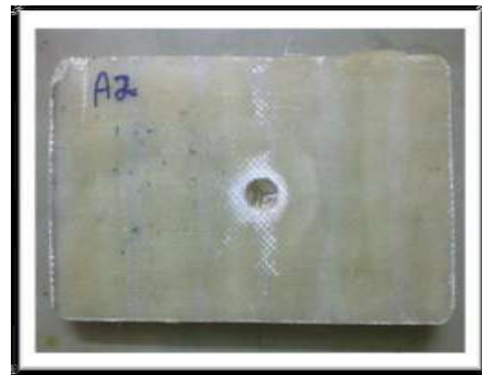
Fig.11 Image of Damage of Sinusoidal Core Top Side
