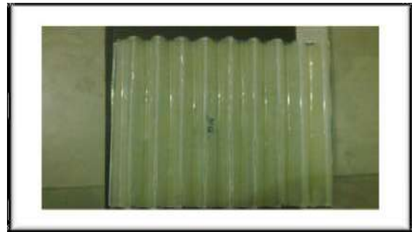
Fig.6 Cured Core Cut to Size
