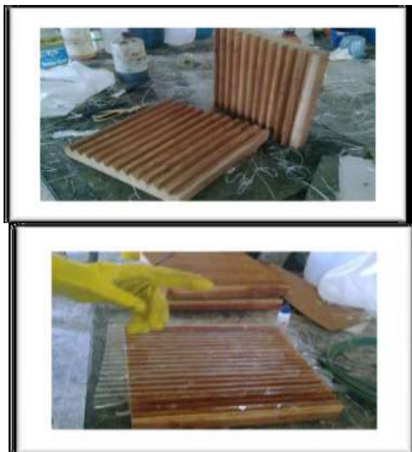
Fig.5 Applying Polythene Sheet
