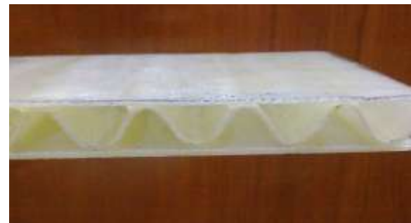
Fig.7 Core Bonded With Face Sheets
